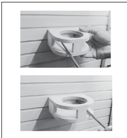
18. Install the cup holder (part I) with ST3.5*25mm screws (2 pcs).
